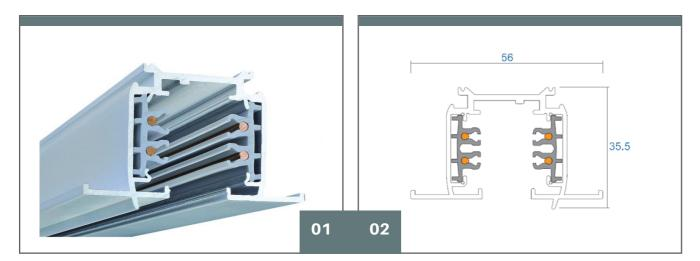
High quality 3-circuit track system for the professional lighting market Suitable for track lights with 3-phase adapters of all major brands A comprehensive range of innovative accessories, like the twisted L and T connectors Maximum freedom to create the ultimate track plan Quick and easy to install No need to adjust the wires after cutting the track Available in white, black and grey
