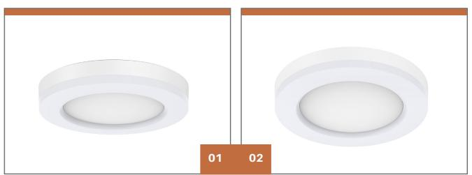
Downward and side lighting creates a uniform light output Interchangeable CCT(3000K+4000K+5700K) with slide switch Dimming: Non-dim, Triac, DALI Optional functions: Emergency, S7 microwave sensor Surface mount / suspended mounting options Life hours > 50,000hrs L70
